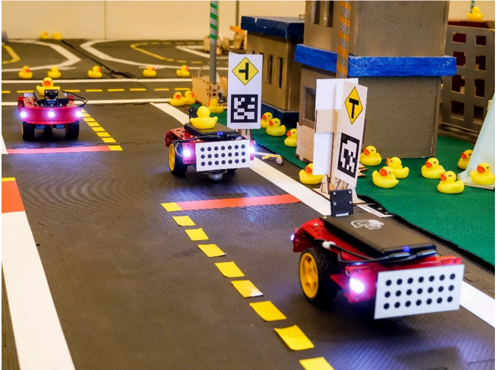
Figure 6.1. A Duckiebot following a lane following in the presence of other vehicles, in a Duckietown with intersections.
