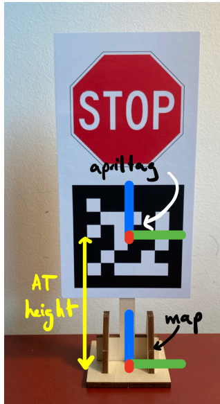
Figure 4.3. Example traffic sign to be used for Apriltag localization. In order to accurately construct your TF tree, please measure the height indicated
